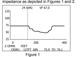
Water inside a cable leaves a recognizable signature of erratic reductions in impedance as depicted in Figures 1 and 2.
