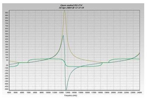
The anti-resonant readings are good, but the resonance readings have the distortion. The distortion shows up at 6 and 18 MHz, and on the left side of the Smith chart. If you want to make plots for the customer, the VIA Bravo is strongly recommended, as the zero crossing distortion of the VIA will cause your customers to ask too many questions.
