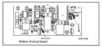
Figure 4. SWR-121 V/U Jumper Locations
