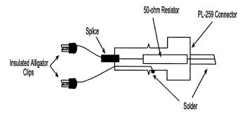
Figure 3 50 ohm accessory connector
