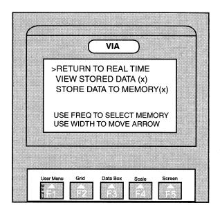
Pressing the WIDTH KEY UP or DOWN will move the left arrow to one of three menu items. A subsequent ENTER key will perform the selected function. Pressing the FREQ key UP or DOWN will cycle through the possible memories. The (x) shown in the second and third menu items will toggle from A to B to C to D and back to A again, or the reverse. This selects which memory will be operated on for the VIEW and STORE functions.
