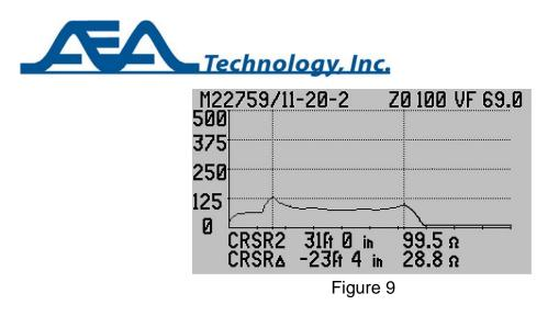
This testing method can also be used to test a coax cable's shield for shorting to the airframe. Simply connect one test lead to the coax cable's shield and the other to the airframe. In some cases that short in intentional for grounding the shield. So the TDR can show a ground is in-tact. However, other cases can be where the cable's insulation has chaffed away creating an unwanted ground.
